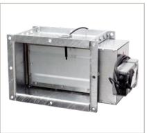
The FläktGroup marine fire damper, MFDA, are tested and type approved according to Solas Class AO and A6O and by most recognized classification societies such as BV, LR and DNV-GL. The damper is certified according to Marine Equipment Directive Module B with certificate nr EUF129-20001899-MED. Our fire dampers can be used on both Marine and Navy ships.
